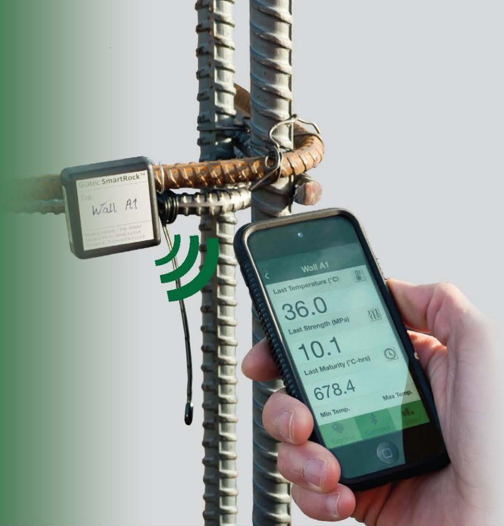
SmartRock™ helps monitor temperature variations in fresh concrete as well as optimize removal time of formwork.
