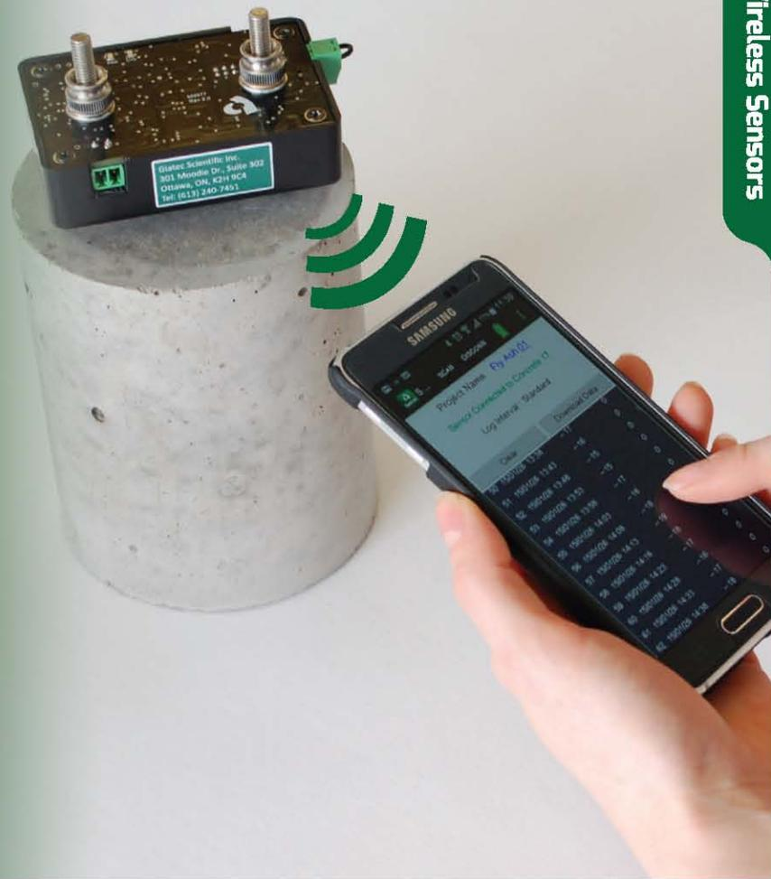
SmartBox™ is a compact wireless device for simultaneous measurement of electrical resistance and temperature.
